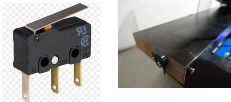
Figure 7 Limit Switch and using Limit Switch in the incline plane
