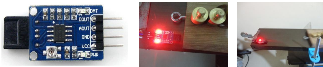
Figure 8 LM 393 IR Sensor and sensing the object and out of sensing the object
